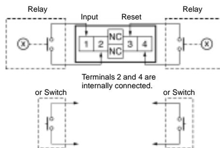
Note: Use Relays and Switches that have high contact reliability because the current flowing from terminals 1 or 3 is as small as approx.  $10 \mu\text{A}$ . OMRON's G3TA-IA/ID is recommended as the SSR.
