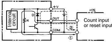
If an excessive voltage is applied to the count or reset input terminals, the internal elements may be damaged. Ensure that the following voltages are not exceeded:
