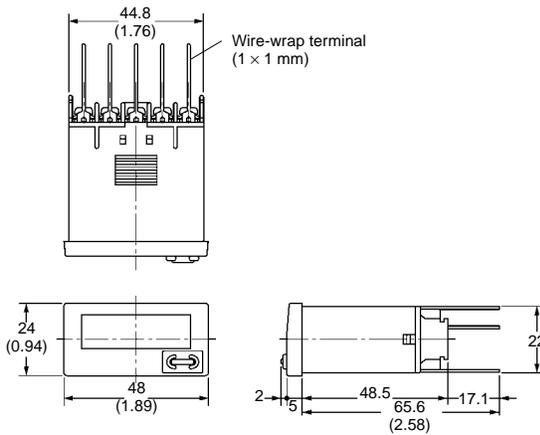
The wire-wrap terminals have a cross sectional dimension of 1x1 mm. Select one of three gauges of wire from the table at right. Also listed in the table is the appropriate wiring hardware
