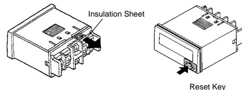
Switch settings on the Counter must be performed before mounting it to a control panel.
