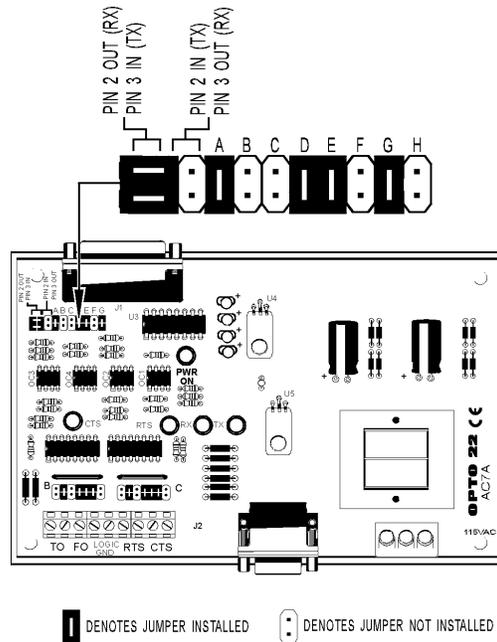
**Figure 2-9: Jumper Settings for Standard Straight-Through RS-232 Cable**
