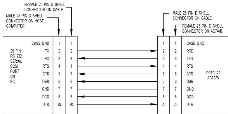
Figure 3-3: Standard Straight-Through 25-Pin to 25-Pin RS-232 Cable
