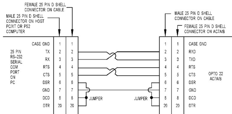
Figure 3-7: 25-Pin to 25-Pin Null Modem Cable Diagram
