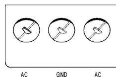
Figure 3-2: Connector Terminal
