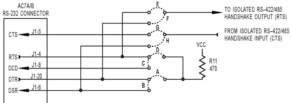
Figure 4-5: AC7A/B Jumpers A through H Schematic
