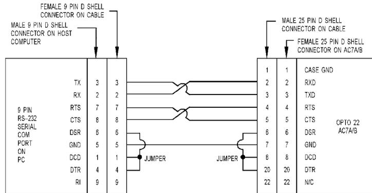
Figure 3-8: 9-Pin to 25-Pin Null Modem Cable Diagram
