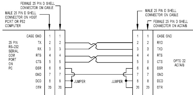
Figure 2-7: 25-Pin to 25-Pin Null Modem Cable Diagram
