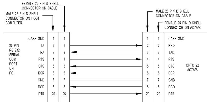
**Figure 2-3: Standard Straight-Through 25-Pin to 25-Pin RS-232 Cable**
