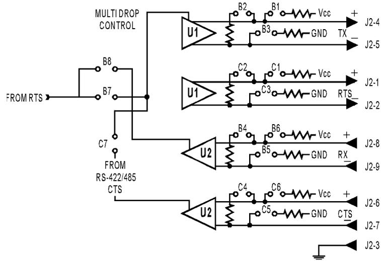
Figure 3-12: Group B and C RS-422/485 Jumper Schematic
