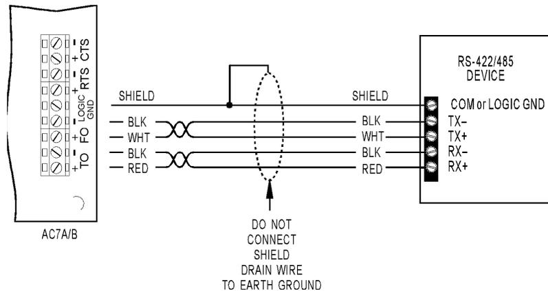
Figure 3-14: RS-422/485 Cabling Diagram (alternative, less noise immune)
