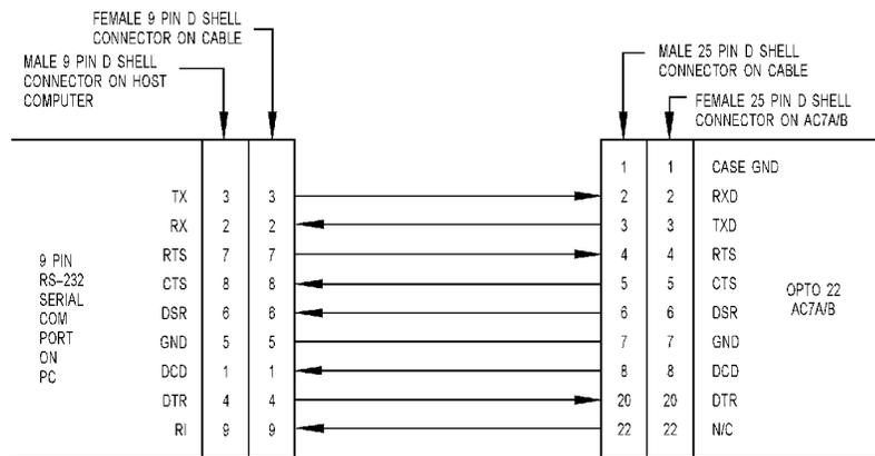
**Figure 2-4: Standard Straight-Through 9-Pin to 25-Pin RS-232 Cable**
