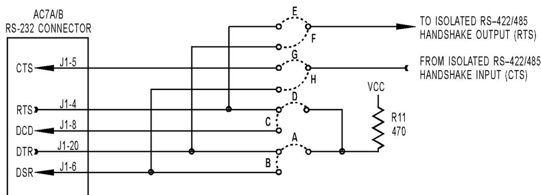
Figure 3-11: AC7A/B Jumpers A through H Schematic
