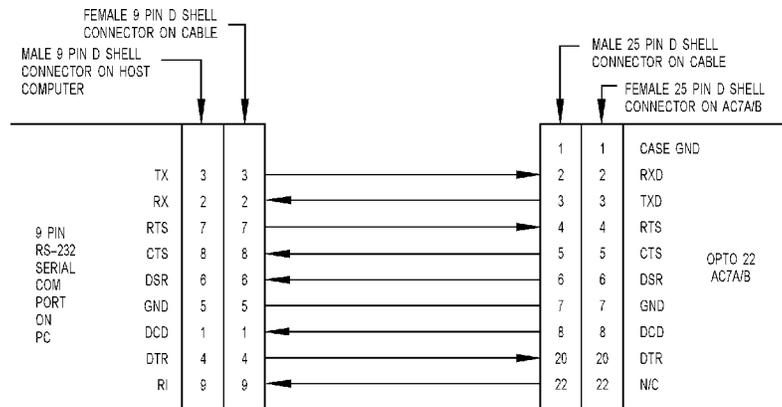
Figure 3-4: Standard Straight-Through 9-Pin to 25-Pin RS-232 Cable
