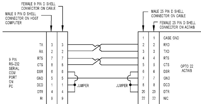
Figure 2-8: 9-Pin to 25-Pin Null Modem Cable Diagram
