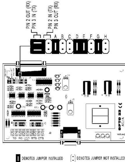
**Figure 3-9: Jumper Settings for Standard Straight-Through RS-232 Cable**
