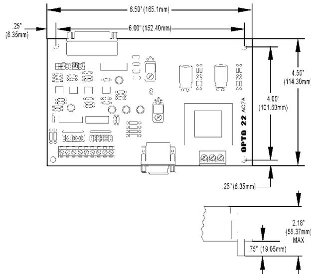
Figure 2-1: AC7A/B Card Dimensions
