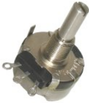
53 Series Industrial Potentiometer, Conductive Plastic Element, Solder lug Terminals, 2 W Power Rating, 250 kOhm Resistance Value
