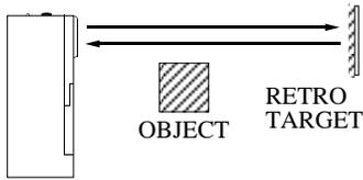
**SBLV1:** visible beam makes alignment very easy, and is the first choice for most retroreflective applications. Not for use in dirty environments; rather use opposed mode or see SBL1 & SBLX1, below. Do not locate retroreflector closer than 6 inches (15cm) from sensor.
