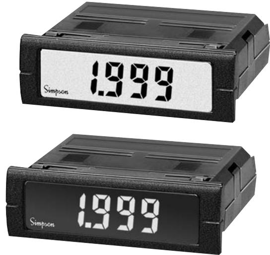
Simpson's Mini-Max Frequency meters provide accurate, stable, frequency indication in a compact, 60mm deep case. Units have a 3-1/2 digit, 0.5" (12.7mm) LCD display and are available with a bright red, negative image backlight option. Display hold is a standard feature. Screw terminal connectors provide easy wiring of power supply and input signal.
