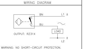
ALWAYS WIRE A LOAD IN SERIES WITH THE SENSOR.
