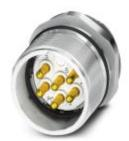
Device connector for front wall, straight, shielded: Yes, SPEEDCON locking, M23, Number of positions: 8+1, Type of contact: Male connector, Solder connection, Seal, axial, Central fixing
