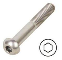
Button Head Socket Screws are designed for light duty with a similar thread design as a Socket Cap Screw although the dome shaped head is wider and has a lower profile than a Socket Cap Screw, presenting an aesthetic appearance to an assembly.
