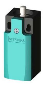
SIRIUS POSITION SWITCH W. INCREASED CORROSION PROT. PLASTIC HOUSING ACC. TO EN50047, 31MM DEVICE CONNECTION 1X(M20X1.5); 1NO/1NC SNAP-ACTION CONTACTS (REPLACEABLE) TEFLON PLUNGER
